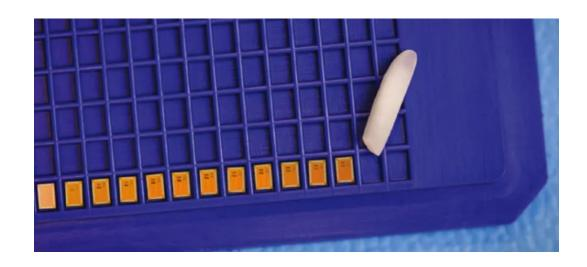
A set of ultra-low-power WiFi radios integrated in small chips, each measuring 1.5 square millimetre
