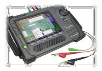
With new enhancements built into the TALAN software interface, users can now also test Internet Protocol (IP) packet traffic on Voice over Internet Protocol phones and systems. Data can be stored and exported to USB or Flash as data files for further analysis, sharing and reporting.
