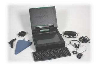
external supply. Its integrated antenna system provides wideband performance from 10 kHz to 26GHz.
